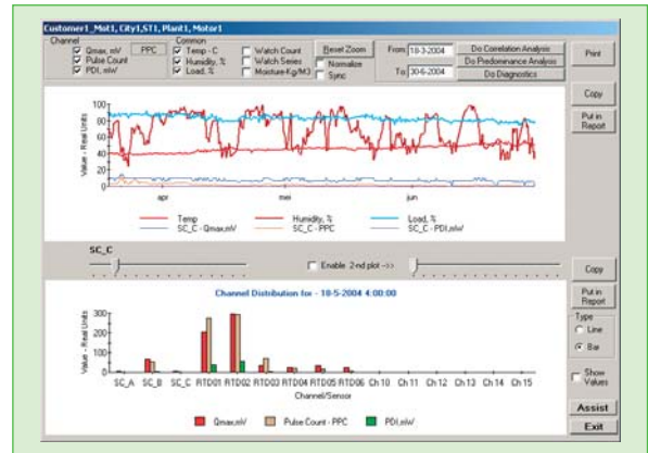
Partial discharge measured for each channel
